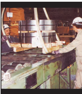
Combined with secutex® protective coating, SpanSet's Web Slings make simple work of lifting sharp edged wire coils (left) and heavy gears (right).
