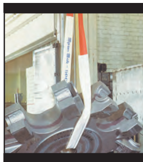
Combined with secutex® protective coating, SpanSet's Web Slings make simple work of lifting sharp edged wire coils (left) and heavy gears (right).
