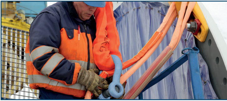
Magnum-X with secutex® clip sleeving to protect against sharp edges.
