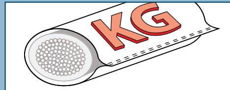
Raised, woven-in load capacity indicator.
