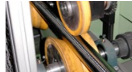
Guide and pressure rolls with exchangeable cores
