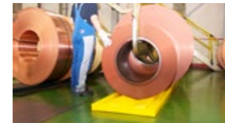
Coil mat with oil drainage channel
