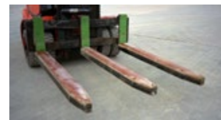
Semi-circular forks for the transport of concrete pipes
