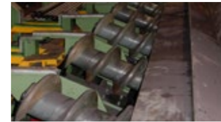
Transport screws for lateral movement
